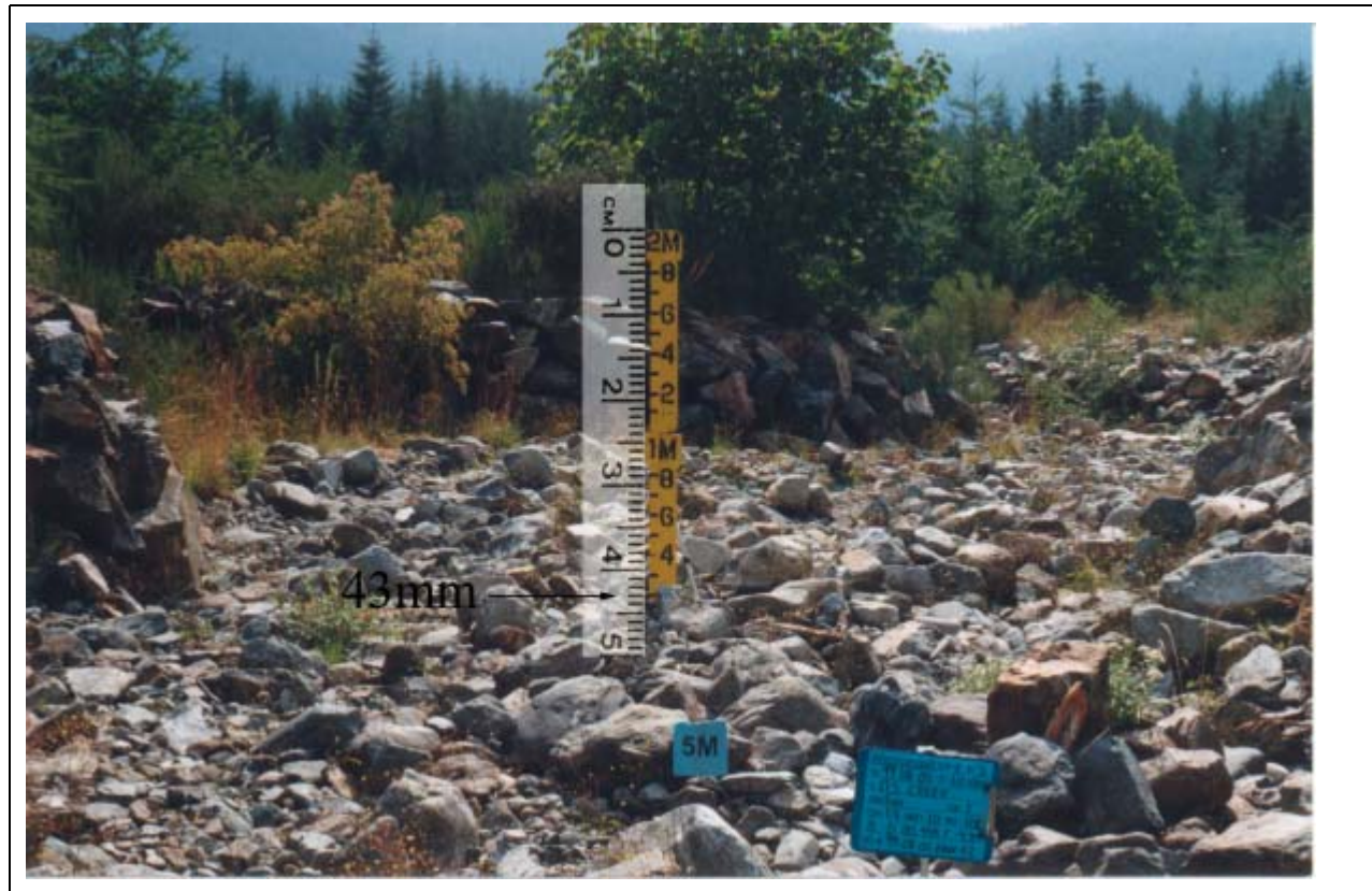
Figure 29. Height of the meter board (mm) for determining the adjustment factor for the master grid. The first clear decimeter marking is the 2 dm. The height of the meter board from the 2 dm to the top is 43mm (Photo Code: 990805-FAN-F1).
