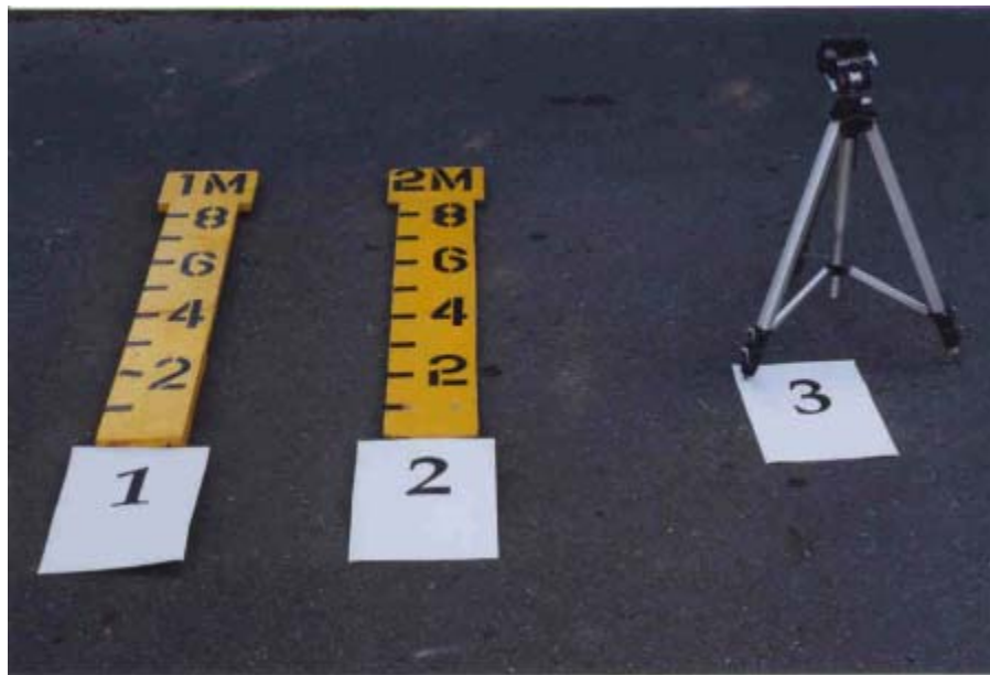
Figure C1 (1-3): Depicts meter board (1), meter board extension (2) and meter board tripod (3).
