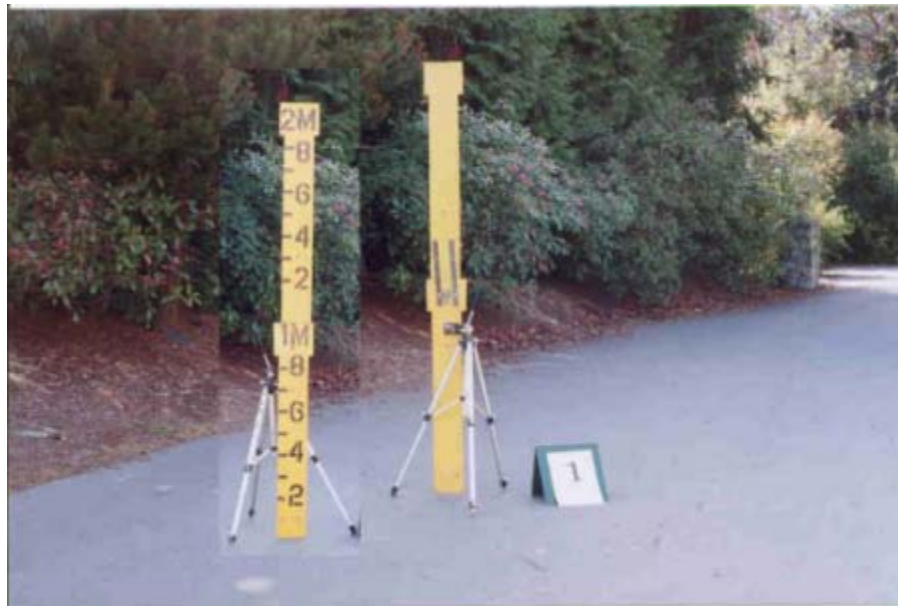
Figure C2 (1): Depicts front and back sides of completed meter board assemblage.
