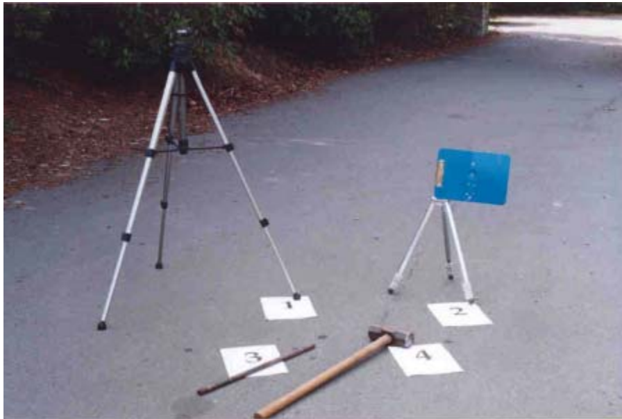
Figure C4 (1-4): Depicts camera tripod (1), data board (2), case-hardened side walk stake (3) and sledge hammer (4).
