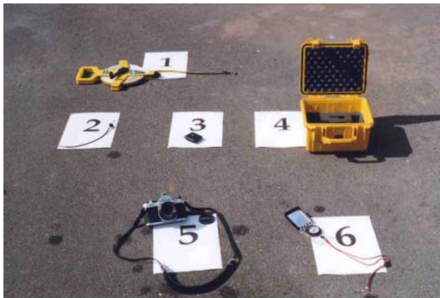
Figure C6 (1-6): Depicts fiberglass measuring tape (1), shutter release (2), camera mount (3), pelican case (4), 35 mm camera with 50 mm lens (5) and compass (6).
