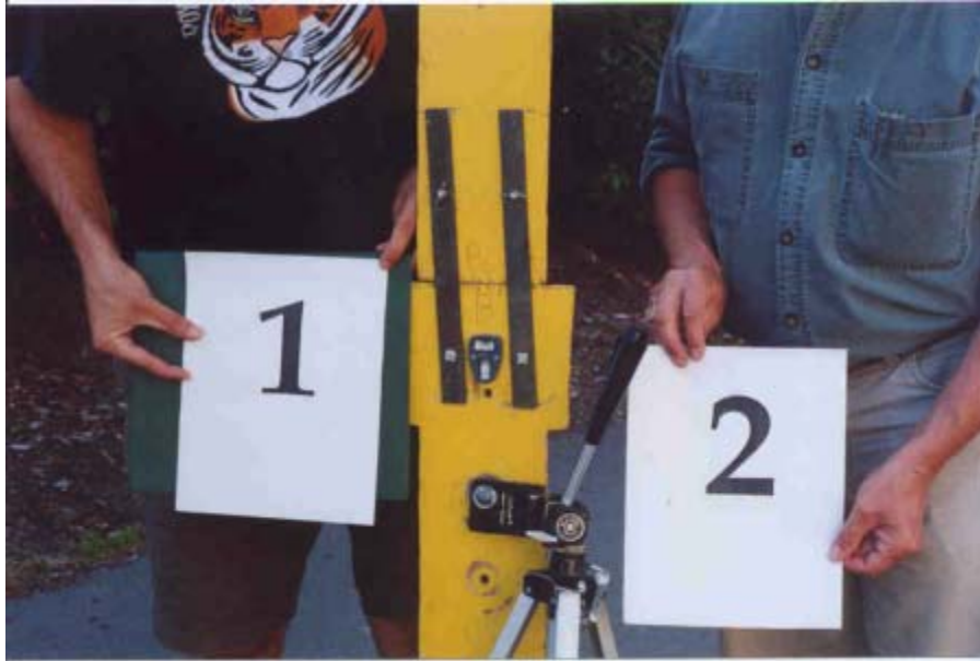
Figure C3 (1-2): Depicts meter board leveling mechanism (1) and meter board attachment mechanism (2).
