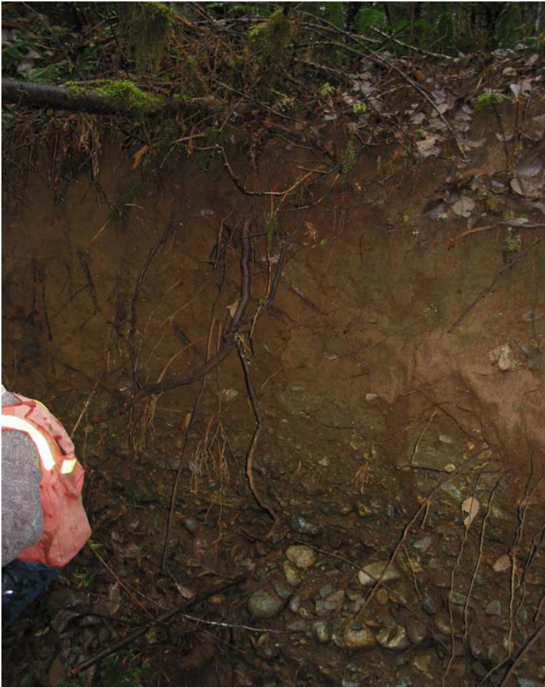
Photo 13: Dry 3m deep test hole near the hatchery. Note the 1m deep overbank sediments over top of gravels and sands.
